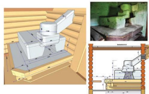
Fig. 5, 6, 7. The house from village Rivnia (1861), transferred to the Museum in 2013—3D model, drawing, 3D model and drawings of furnace
