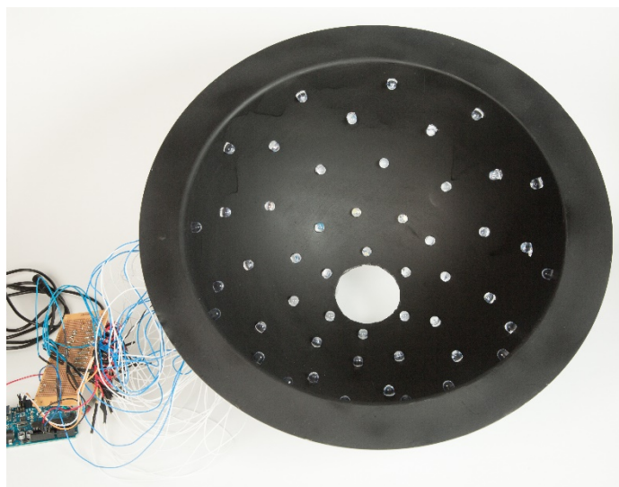
Figure 8. Inside of the large sphere showing the 50 LED lights. Each light is a 10 mm super bright LED and can be independently controlled by the Aduino Uno microprocessor.
